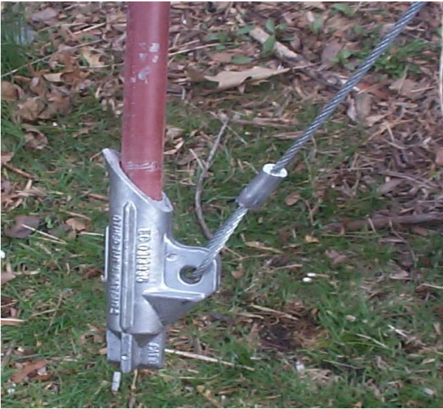
Drive Rod inserts into Anchor Head
