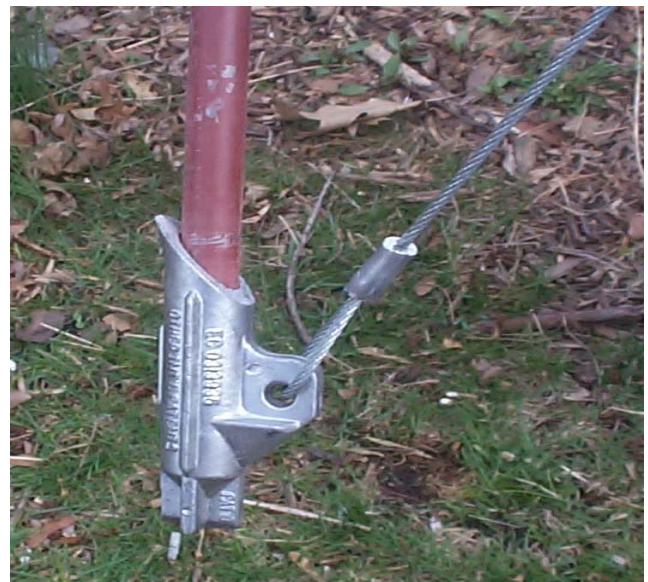
Drive Rod inserts into Anchor Head
