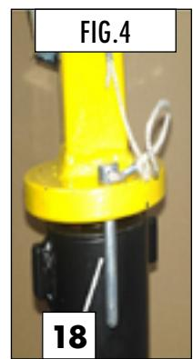
**STEP 1.** Attach the Hook with Chain (8) to the correct maximum weight capacity on the Boom (1) by repositioning it as needed and replacing the Bolt and Lock Nut. The weight of the cargo must fall below the maximum weight setting chosen (500 Lbs., 750 Lbs., and 1,000 Lbs.).
