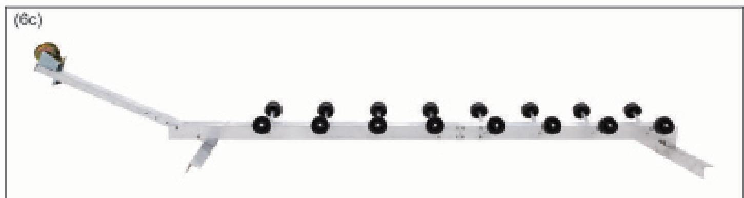
**Step 7:** Attach the remaining two wheels (I) and roller (J) to the end of the rear beam using the roller rod (F) and R clips (S). Slide the roller rod into one hole, through the roller fit into the space in the beam, then through the second hole. Fit the wheels onto each end, and secure with R clips, bending with a pliers to secure.
