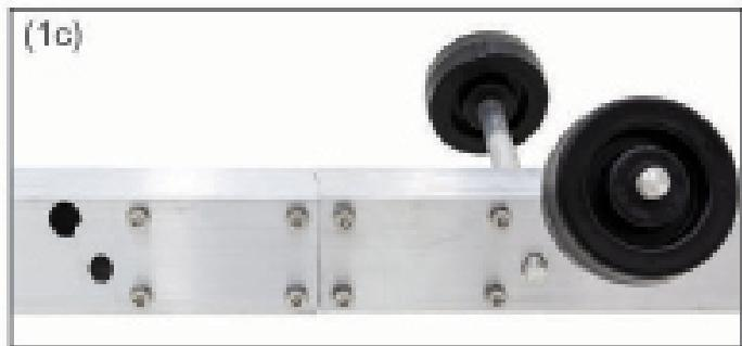
**Step 2:** Install the legs (C) onto the center beam (A) using the M10x130 bolts (G), washers (J), and nuts (K). Tighten securely with 17mm wrenches.
