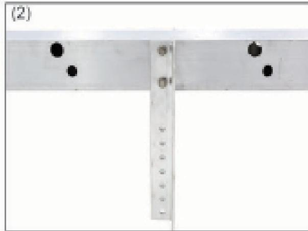
**Step 3:** Install the angle foot (D) onto the legs (C) using the M10x25 bolts (2), washers (J), and nuts (K). The foot may be set to the adjustment that best suits your needs. Tighten securely with 17mm wrenches.
