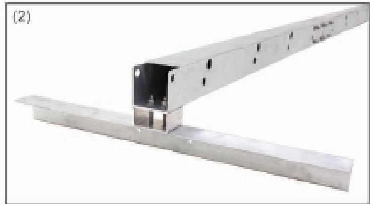
**Step 3:** Attach the winch post (C) to the front beam (A) using the M10x130 bolts (M), washers (Q), and nuts (R). This post may be set to the adjustment that best suits your needs. Tighten securely with 17mm wrenches.
