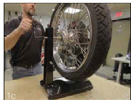
**STEP 2.** Install and adjust the truing arm so that it is just shy of touching the wheel. Slowly spin the wheel in either direction. Adjust the spokes where the arm touches the tire or appears to drift away. See FIG 2a, 2b and 2c.
