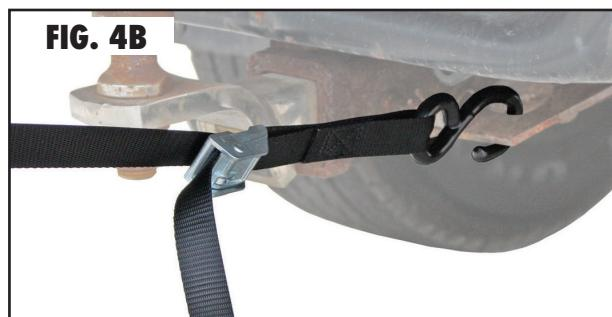
Hitch chain loop tie down point recommended for full width ramps.
