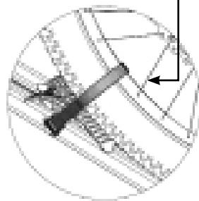
When the bike's tire is against the wheel cradle, press the button on the wheel cradle to secure it firmly.
