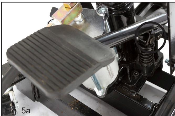
**Step 6.** Install Handle (5) to handle bracket on Jack. Secure Handle with bolt and nut.
