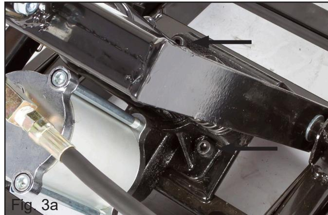
**Step 4.** Remove nuts from Lock Support Bar (3) and install to side lock bars. Apply nuts and tighten with 1/2" wrench. **\*NOTE: Angle of Lock Support Bar (3) should be running away from Jack platform\***
