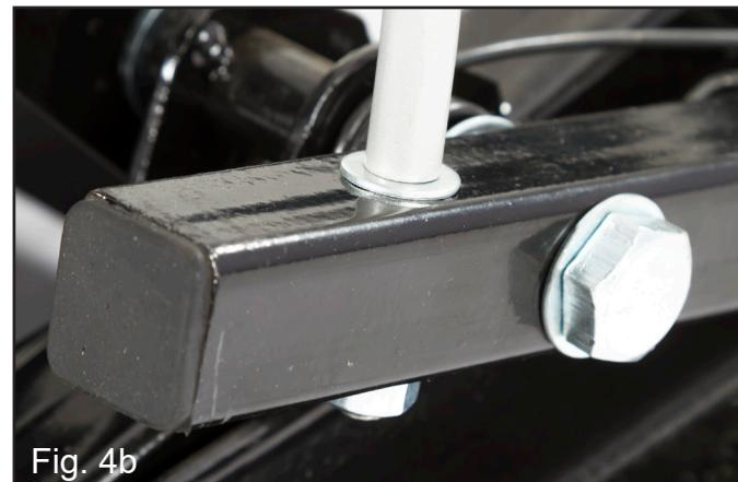
**Step 5.** Remove pins from Foot Pedal (4) and install to Air Pump Assembly. Re-apply pins.
