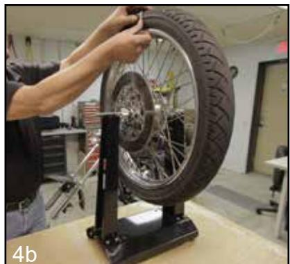
5. Add or remove the appropriate amount of weights to counter balance the wheel. When the wheel stops rotating on its own, then it's balanced.
