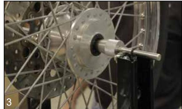
4. Check the balance by turning the wheel 90 degrees either way and let go. If the wheel is out of balance, the heavy side will rotate to the bottom. Once the wheel has stopped moving, mark the top or light side.
