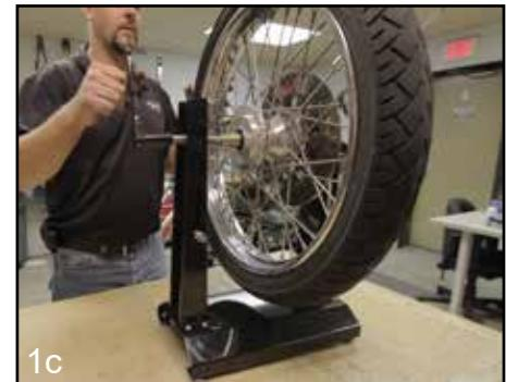
2. Install and adjust the truing arm so that it is just shy of touching the wheel. Slowly spin the wheel in either direction. Adjust the spokes where the arm touches the tire or appears to drift away.
