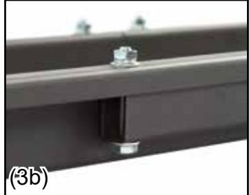
**Step 4.** Connect the kickstand plate to the track plate assembly using the M8x15 flat head bolts, washers, lock washers, and nuts. The kickstand plate may be placed in five different positions on either side of the track. Attach the plate in the appropriate position for your motorcycle's kickstand. Tighten securely. Place the two safety pins in the slots on each end of the track plates.
