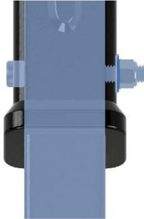
Do NOT put a washer on the head of the bolt - the washer goes on the nut end. Insert the bolt into the hitch pin hole and ensure the bolt head recesses into the hitch pin hole until it stops against the MotoTote tube inside the hitch. This is critical to eliminating any shake by clamping the square tube to the hitch. Then using an allen wrench and a socket wrench, tighten until the connection to the hitch is solid with no play. Do not over-tighten.
