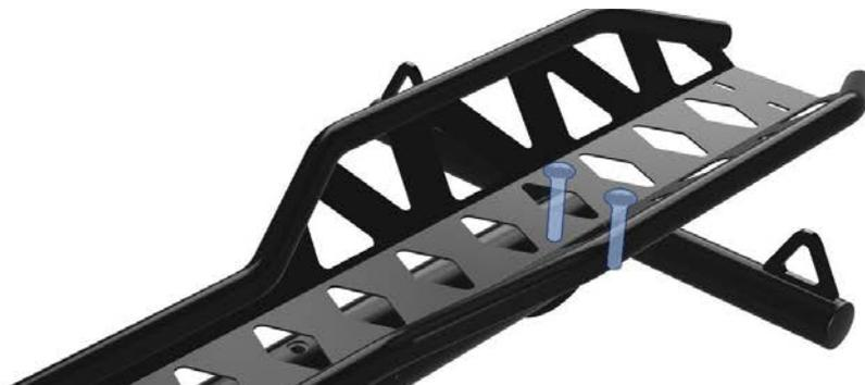
Now, on the opposite side of where you selected to put the wheelstop, insert the rear tie down arm into the slot and lay down the tire track on the platform. align with the two holes. Insert the two bolts into the tire track and through the holes. Put on the nuts and washers then tighten snugly to minimize rattling Do not overtighten. NOTE: The tracks look different but procedure is the same.
