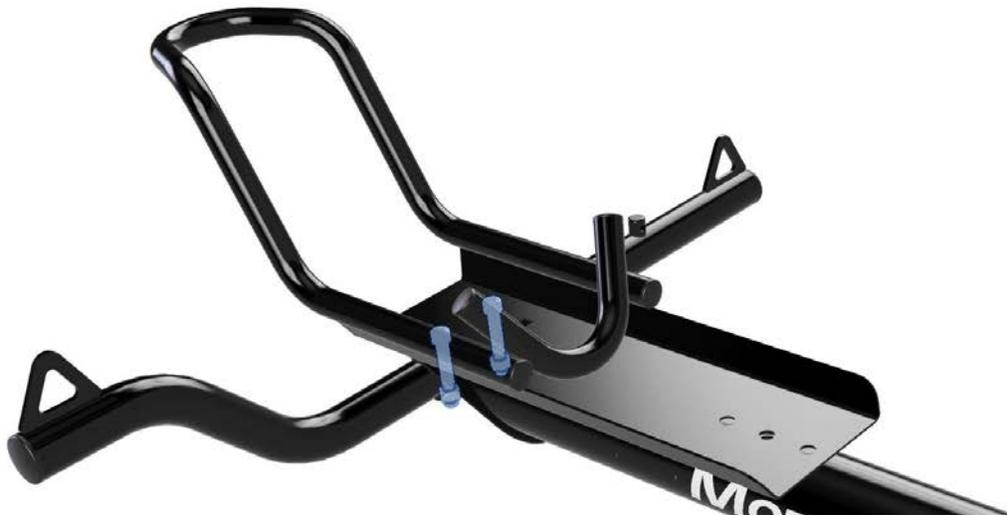
Place the front tie down arm in the slot of the platform, making sure the curved section is facing outward. Lay down the wheelstop onto the platform and align with the holes then insert two bolts to the desired placement (there are three positions dependant on your motorcycle length). Put on the nuts and hand tighten only for now (this is to ensure alignment of loading ramp in Step 4).
