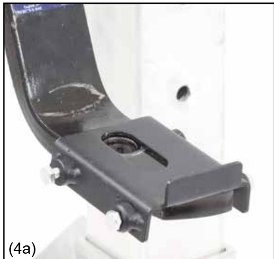
**Step 5.** Install carrier to hitch adapter and stabilizer with M16x85 bolt (7), M18 washers (8), M18 lock washer (9), and M18 lock nut (10). Secure with 1" wrench.
