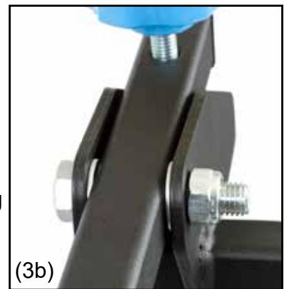
**Step 4.** Install stabilizer (5) to vehicle hitch adapter. Tighten side bolts with 10mm wrench.
