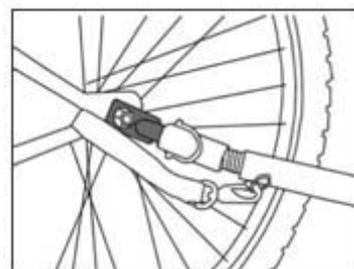
Position the trailer behind the bicycle so that the female connector on the tow bar can slide over the male connector on the hitch. Lock these connectors in place with the cotter pin. Loop the black safety strap around the bike frame and attach the snap swivel to the D-ring on the tow bar.
