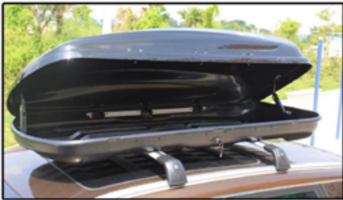
**Step 2.** Hook the u-bolt to the bottom of the crossbar to link the roof box.
