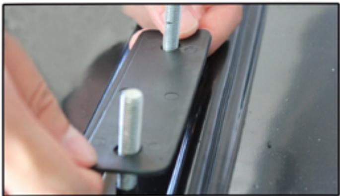
**Step 4.** Change bandage parts to strap mounts. The strap loop faces inward.
