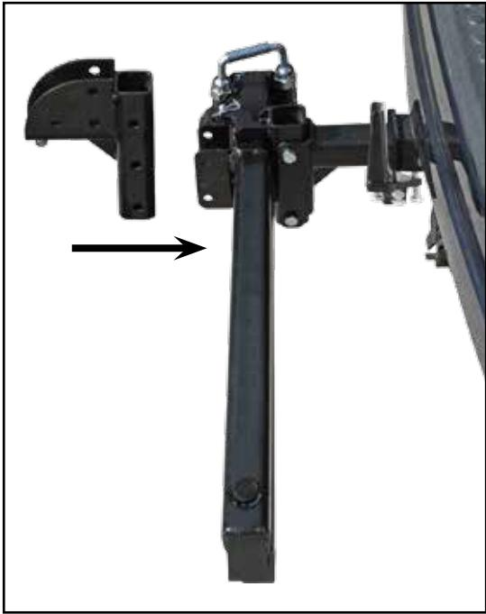
**Step 4.** Bolt in place at the desired drop with two nuts and bolts. Secure with a 19mm wrench.
