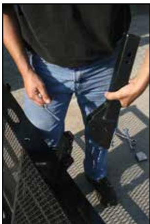
**Step 2.** Slide the carrier into the carrier bracket and lock in place with a lock pin.
