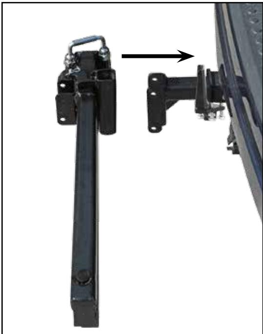
**Step 2.** Bolt in place using two nuts and bolts. Secure with a 19mm wrench.
