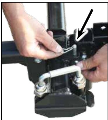
**Step 2.** Pull the latch handle upward.
