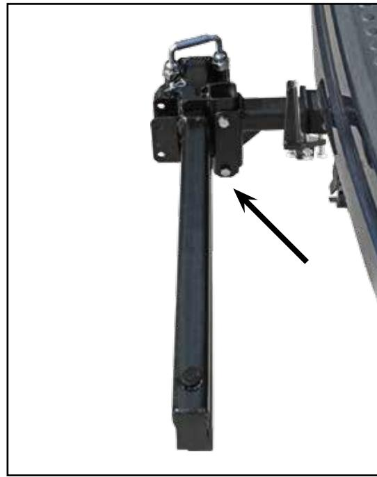
**Step 3.** Align the Carrier Adapter (B) with the Swing Arm (A).
