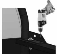
C. Install the hexagon bolt through the spring washer, flat washer, hole of truck rack, and the predrilled hole in the truck. Secure with the mounting plate.
