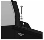
B. Drill a 12.5mm hole at the position of round hole in the upright.
