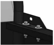
**Step 3.** To install the rear portion of the cargo truck rack on the truck bed, repeat the above steps.
