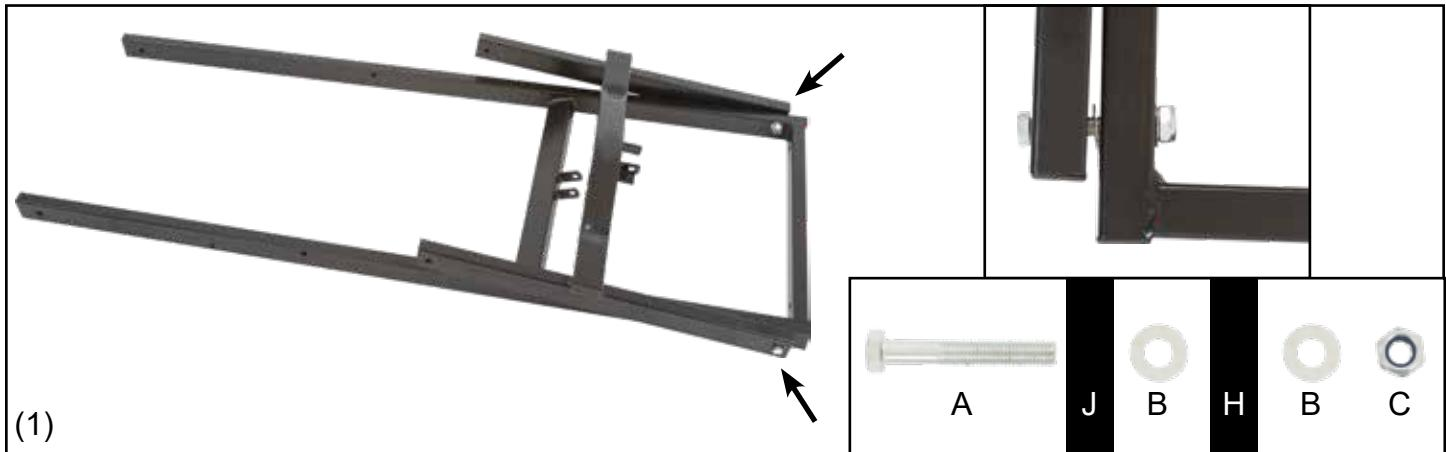
**Step 2.** Install both swing arms (L) to the base (H) with two M10x65 bolts (A), four washers (B), and two nuts (C).
