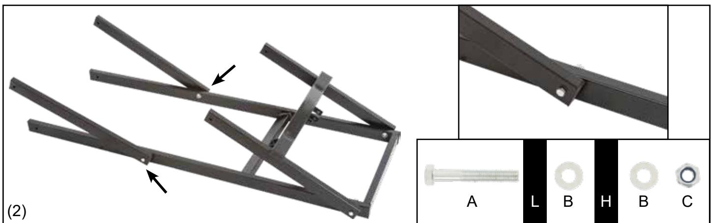
**Step 3.** Install the support bar (I) to the jack base (J) and both swing arms (L) with four M10x65 bolts (A), eight washers (B), and four nuts (C).
