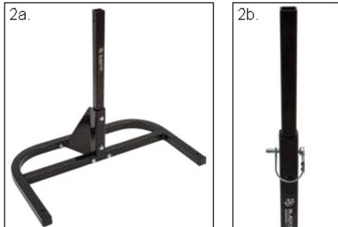
**Step 3.** Assemble the handle mechanism. Connect the support brackets (G, H) to the inner support tube (D) using two M6x45 bolts (K) and nuts (M). Hand-tighten until the assembly is complete. Connect the blockers (J) to the support brackets using one M6x45 bolt (J) and nut (M). Connect the handle (B) to the support brackets using the shoulder bolt (L), and nut (M). When assembly is complete, tighten hardware with wrenches.
